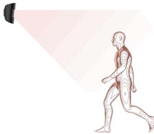
The detector must be installed at 2.4 meters without obstruction to its view. For example, in a corner where the view will not be blocked by a closet or other furniture on which a pet can climb.
