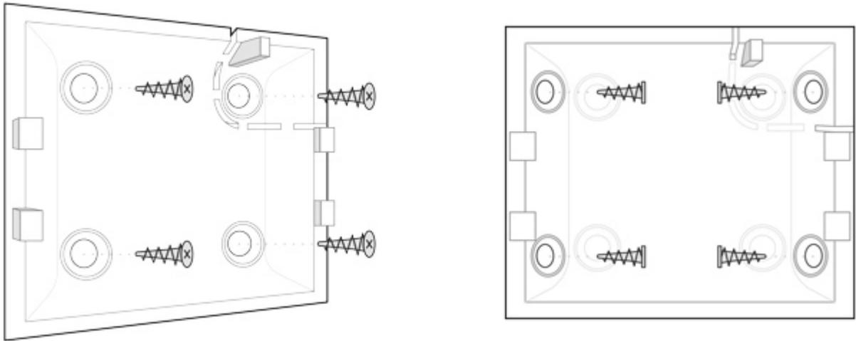
8. Place the detector on the SmartBracket mounting panel.
